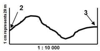
Vertical Exaggeration (VE) of the cross-section is 5 times
