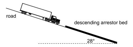
Which arrestor bed, ASCENDING or DESCENDING, will be able to stop the truck in a shorter distance?
