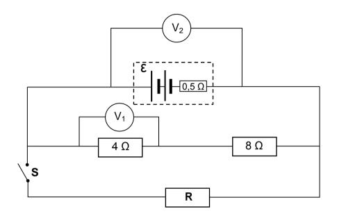
8.1 The three external resistors are ohmic conductors.
