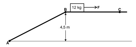
The magnitude of the constant frictional force acting on the block while moving from point **B** to point **C** is 42 N LARGER than the magnitude of the constant frictional force acting on the block when it moves from point A to point B.
