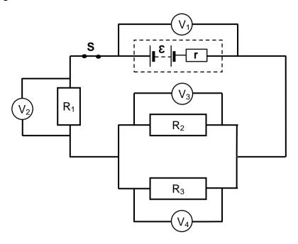
Which ONE of the following equations represents the reading on voltmeter  $V_1$  in terms of the readings on the other voltmeters?
